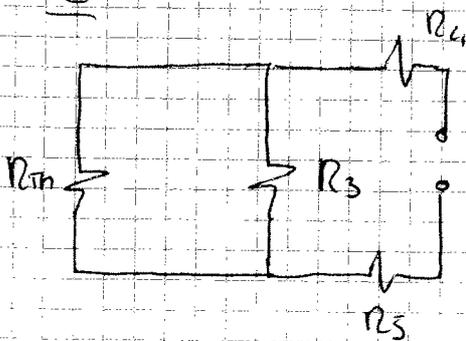
$$R_{EE} = R_4 + R_5 + \left( \frac{1}{R_{TH}} + \frac{1}{R_3} \right)^{-1} = 14,686 \text{ }\Omega$$
