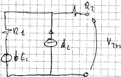
$$V_{TH} = -E_1 + R_1 \cdot I_2 = -20 \text{ V}$$
