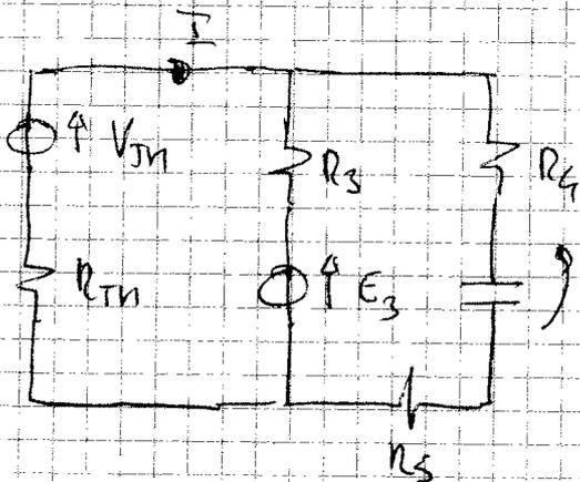
$$I = \frac{V_{TH} - E_3}{R_{TH} + R_3} = -5 \text{ A}$$
