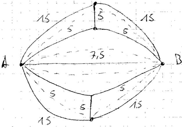
$$R_D = R_A \cdot R_B \left( \frac{1}{R_A} + \frac{1}{R_B} + \frac{1}{R_C} \right)$$
